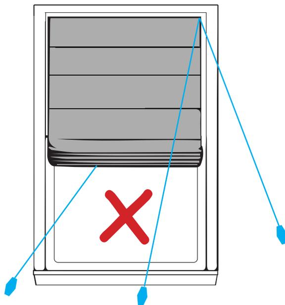
Avoid pulling the cord forward or across the front of the blind or on an excessive angle to the side of the blind. This will cause the cord to rub on the metal cord lock pulley and eventually the cord will fray over time.
