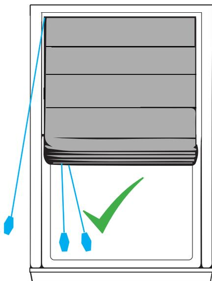
Pull cord on slight angle to side of blind or straight down when opening and closing blind.
